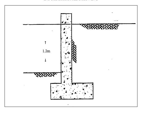
"Retaining Wall" means any structure other than a building wall separating areas of land having a difference in finished grade in excess of 1.2 m.
