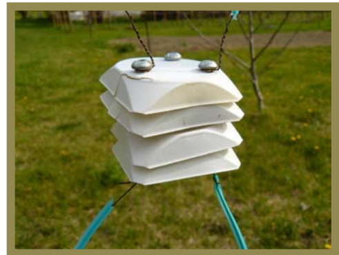
iButton temperature data logger weather shield
